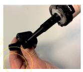
sealant using the retained wipe. You can also usw white spirits or panel wipe to clean off excess if you have accidentally smudged or over applied sealant. Please allow 24 hours to cure fully before attaching any awning or roof rack etc. Dispose of any unused products responsibly.
