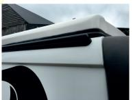
Our Vamoose rails use a standard 6mm x 6mm Kador Strip to fasten any industry standard awning to your van, we also manufacture a universal bracket to install most Fiamma wind out awnings to our Combi Rails.
